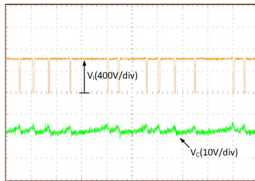
Figure 16. Amplified waveforms of the input voltage of the inverter bridge and the Z-source capacitor voltage corresponding to Figure 15.
