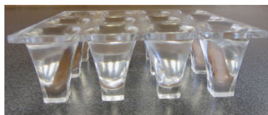
Figure 17. Schematics of a solar concentrator utilizing total internal reflection (TIR) in order to guide the incoming solar radiation to the active solar cell parts (a) and actual concentrator element array made of polyurethane (b) [69].
