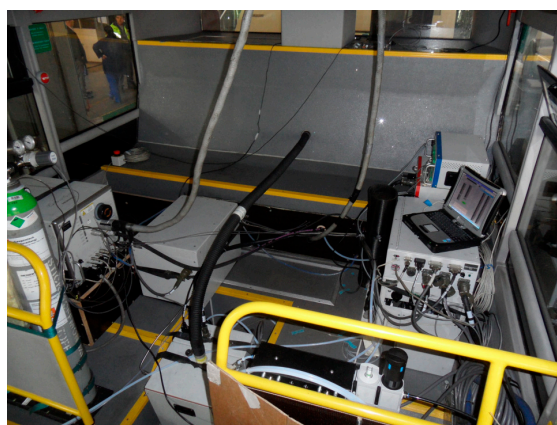
Figure 3. Installed Portable Emissions Measurement System (PEMS) for gas and PM 10 measurements on the DE5 bus.
