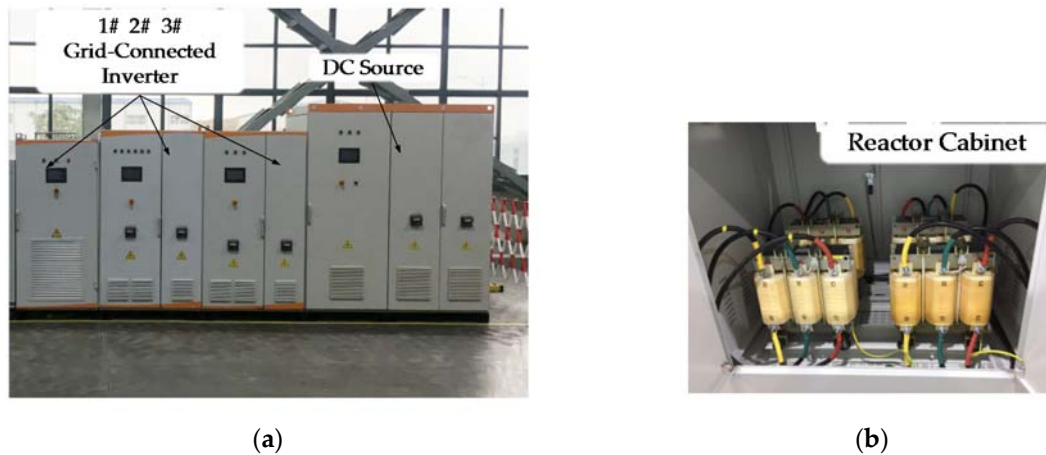
Figure 20. Experimental platform: (a) Three grid-connected inverter and DC source; (b) reactor cabinet to simulate the grid impedance.
