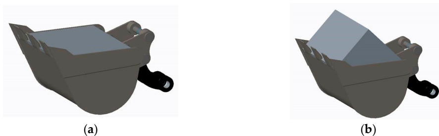
Figure 6. Bucket full of load: (a) full; (b) heaped according to CECE 2:1.
