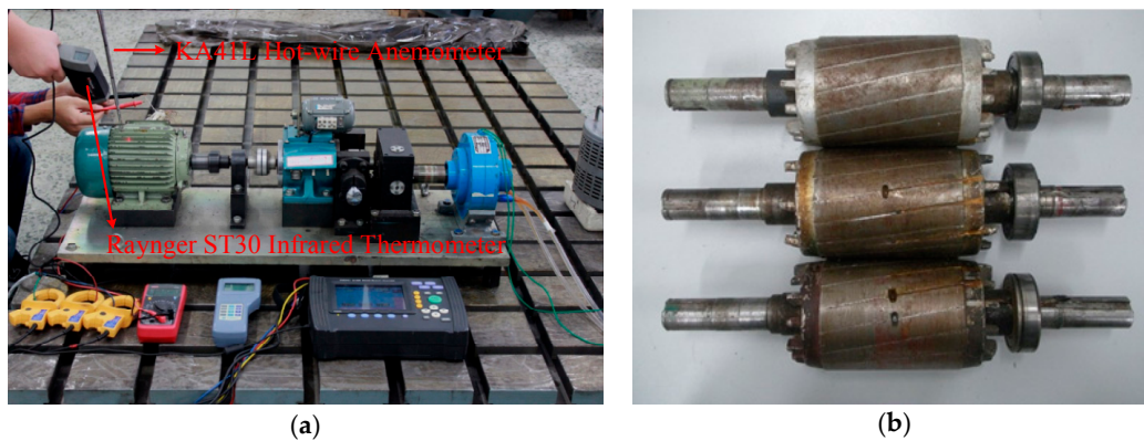
Figure 1. The laboratory test setup and the broken bar rotors: (a) The laboratory test setup; (b) the broken bar rotors.
