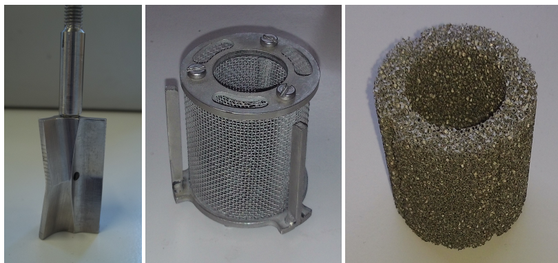
Figure 1. Experimental device. From left to right: gas-inducing impeller, basket, and foam block.
