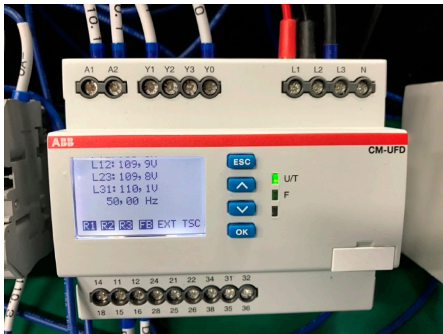
Figure 27. Normal operation of relay.
