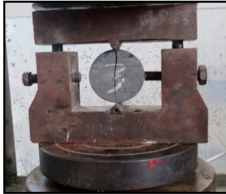
Figure 9. Point load splitting testing of gangue block.
