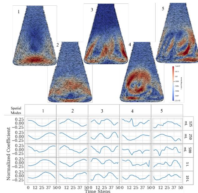
**Figure 4:** Spatial modes for the 5 main modes and normalized time coefficient curve for each mode/scale.
