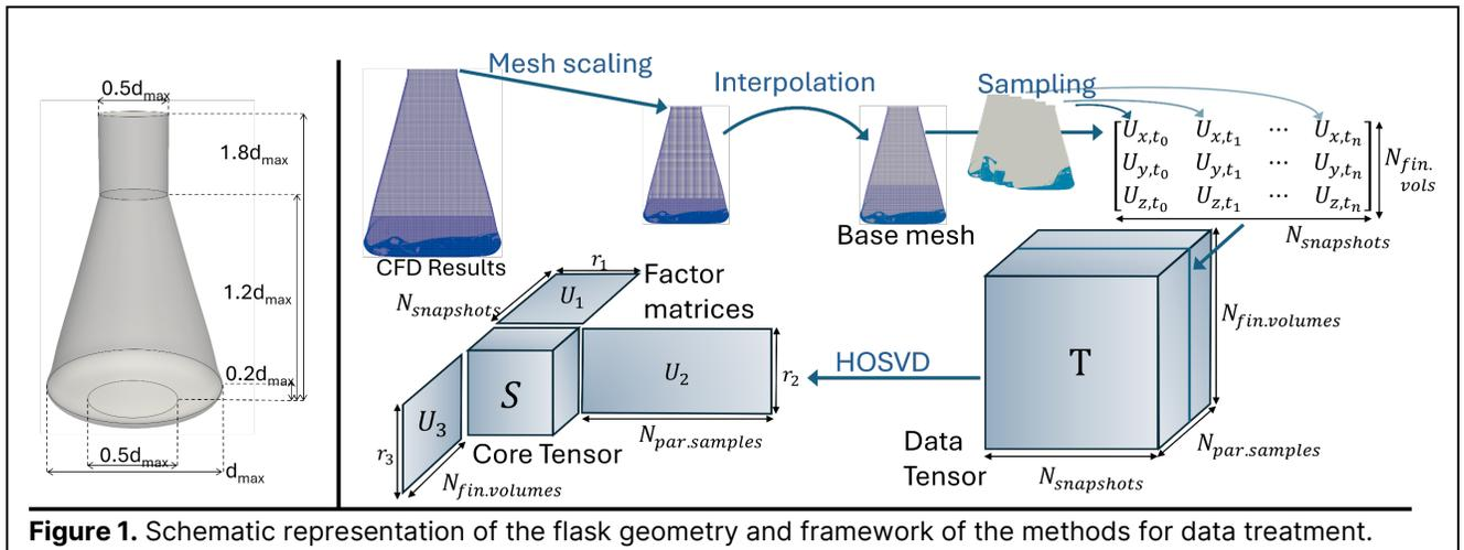
**Figure 1.** Schematic representation of the flask geometry and framework of the methods for data treatment.
