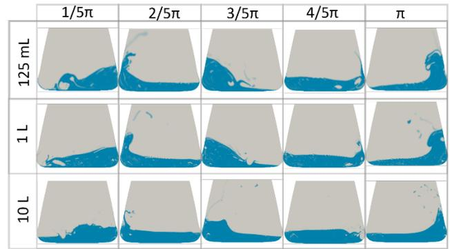
**Figure 2.** CFD results for different flask sizes, with the regions of water volumetric fraction greater than 0.95 painted in blue.
