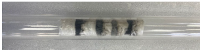
Image 1. Laboratory-scale DFM packed reactor employed.
