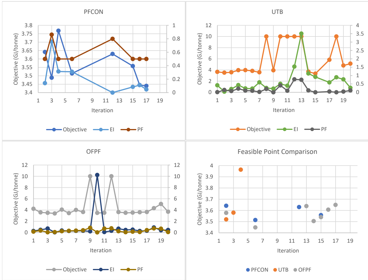
Figure 3: Comparison of objective function, expected improvement, probability of feasibility, and feasible solution progress by iteration. Missing iterations failed to yield a sample point during sample point selection.
