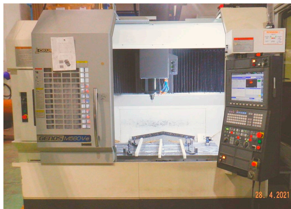
Figure 5. The CNC machining center with the integrated controller.
