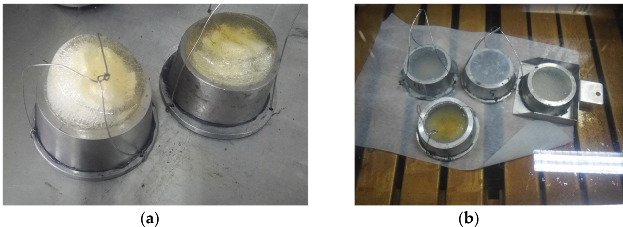
Figure 14. (a) Unstable polymerization of conventional epoxy resins. (b) Stable curing of the modified sealants.
