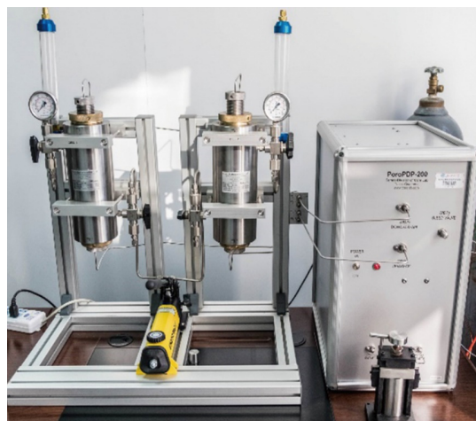
Figure 2. Pulse Decay Permeameter-PDP-200.
