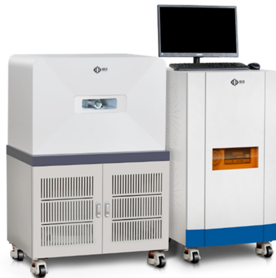
Figure 3. MesoMR23-060H-I instrument for LF-NMR experiments.
