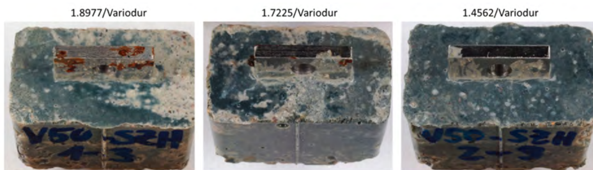
Figure 6. Steel/Variodur specimens after hydrating for 28 days.
