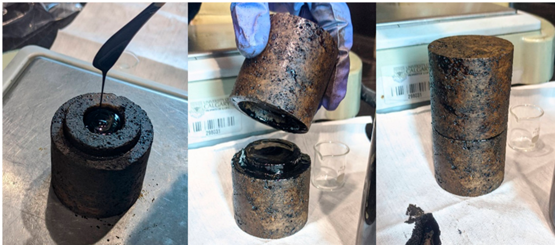
Figure 2. Photographs of an oil-saturated core plug being filled with oil and capped.
