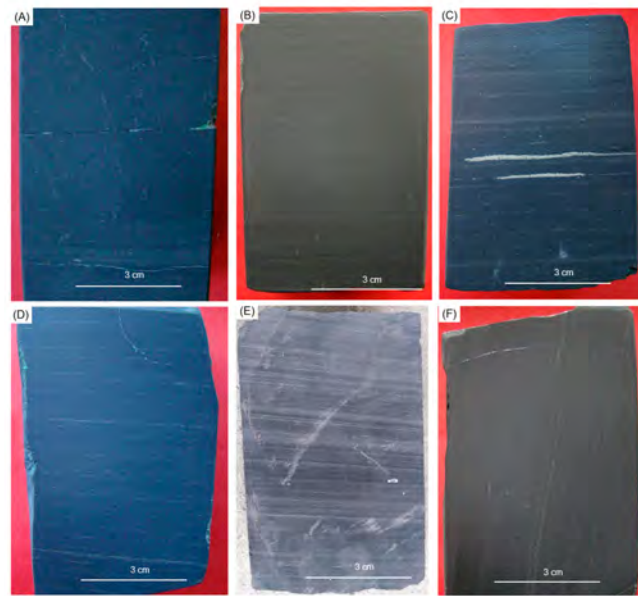
Figure 7. Core and outcrop photos showing general characteristics under the naked eye of shale with various depositional structures in the Wufeng–Longmaxi shale in the Sichuan Basin of southwestern China. (A) PL, with weakly linear lighter color banding occurring alternated with darker layers (sample number 8-31, Longmaxi Formation); (B) GL-C, the colors of the adjacent beds often show a slight differences (sample number 4-2, Wufeng Formation); (C) GL-SC (sample number: 9-19-1, Longmaxi Formation) and (D) GL-SC (sample number 10-12, Longmaxi Formation), and the shale has a distinct “striped” appearance of alternating lighter and darker layers as well as intermittent bright calcite beds; (E) IL (sample number 2018-12, Longmaxi Formation) from borehole Ning 212, and paler beds alternate with darker beds; (F) SB (sample number 5-29, Wufeng Formation) from Shuanghe outcrop in Changning County, and the shale is massive and shows no obvious lamination, bedding or fissility.
