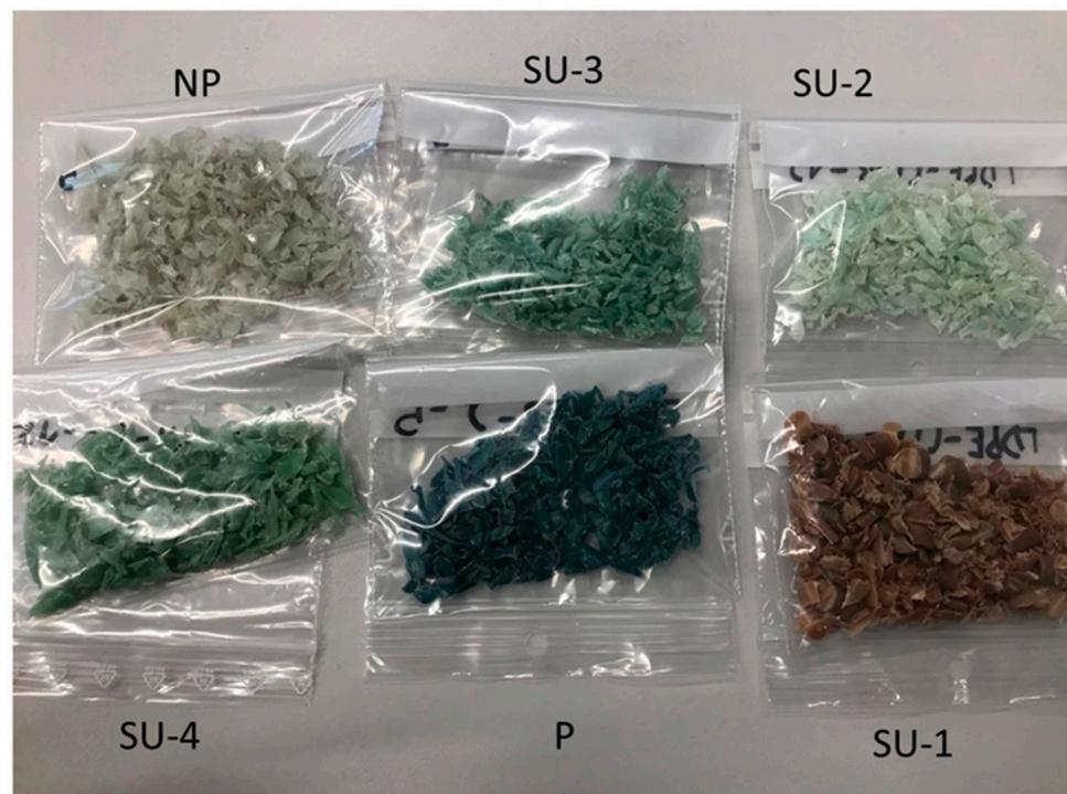
**Figure 5.** The recyclates of the six scaled-up samples after extrusion.
