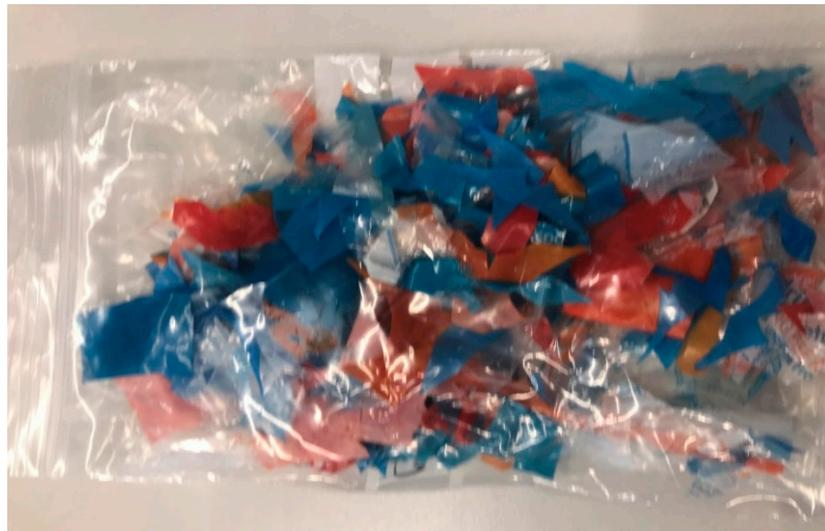
Figure 1. Shredded LDPE samples for the washing experiment.
