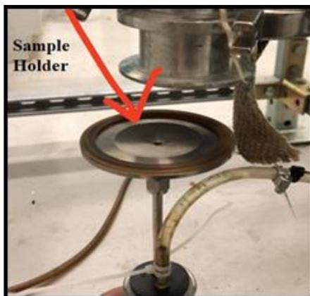
Figure 1: Specimen holder in the quartz reactor.
